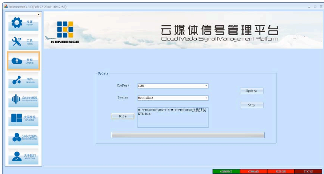
Figure6.3.13 Select serial port, upgrade device, upgrade file
