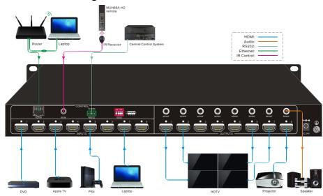
Figure 3-1 Connection diagram
