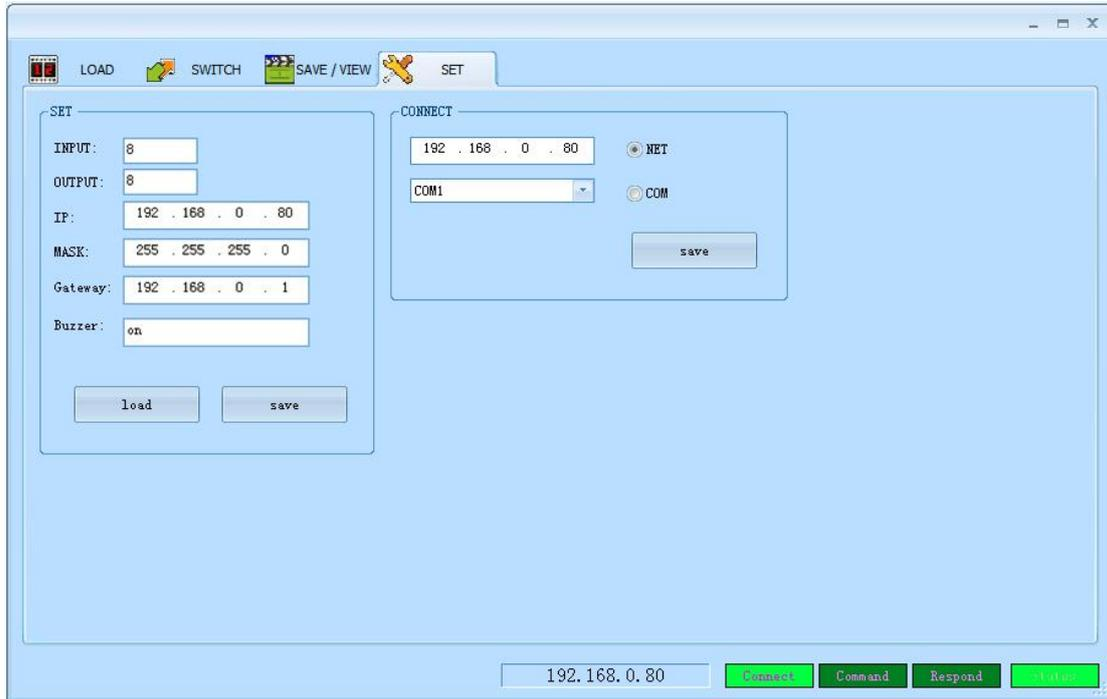
Notice: It's necessary to configure the PC's IP when we use LAN port control mode. See figure 6.3-4. The factory default IP address is 192.168.0.80 .
