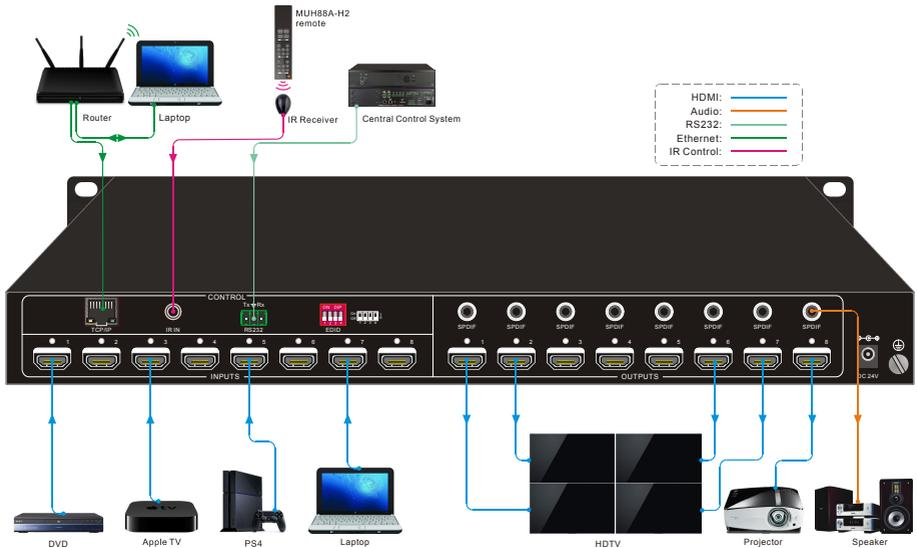
Figure 3- 1 Connection diagram
